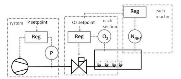
Figure 4. The idea of aeration control using online measurements of ammonium nitrogen concentration; Reg-regulator, P - flow measurement, O2 – oxygen probe, NNH4- ammonium nitrogen probe
