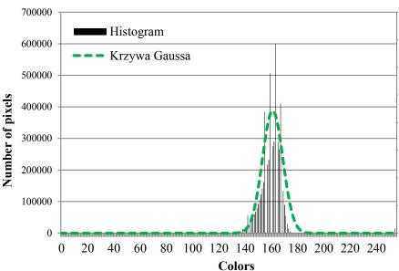
Fig. 2a. shows that the structure is homogeneous with a small number of point defects, which reflect the characteristic lines of the histogram. Its small blurring indicates the high homogeneity of the layer. The largest number of counts in this case is in the range 140-170.
