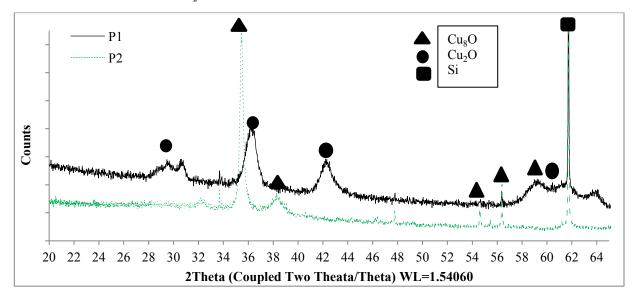
As the XRD diffraction graphs show, the structures differed significantly, indicating the influence of the preparation method. On the basis of the position of the diffraction line, it was found that they originated from phases  $Cu_2O$  and  $Cu_8O$ . Several researchers also reported  $Cu_8O$  in their study (Yonglong 2014; Guan, Hashimoto, Kuo 1984). Table 3 shows the phases detected, grain size, and the crystallinity and amorphicity of the samples.
