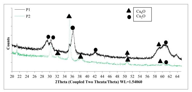
Figure 3. XRD spectra for Cu<sub>2</sub>O samples deposited on silicon
